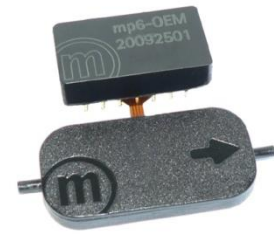
mp6-OEM driver in size comparison to the mp6 micropump
